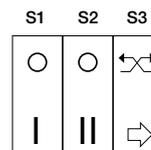
S3 switch activates the "Free cooling" (Bypass) mode, which stops alternate flow and keeps the fan in "extract-only" or "intake-only" mode, to avoid the heat exchange when necessary. To set the "extract-only" mode or "intake-only", place the integral jumpers as per fig. 20A-20B). The front cover LED indicates when the Free cooling mode is on.
